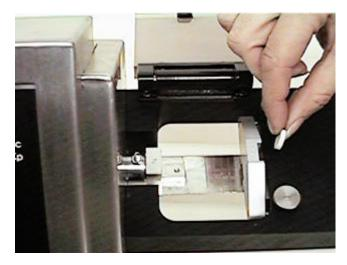
Place the Tablet or Oblong into the Thickness Jaw. Surely the coorect thickness will be measured, no matter of shape and size of sample due to the desing of the Jaw.
