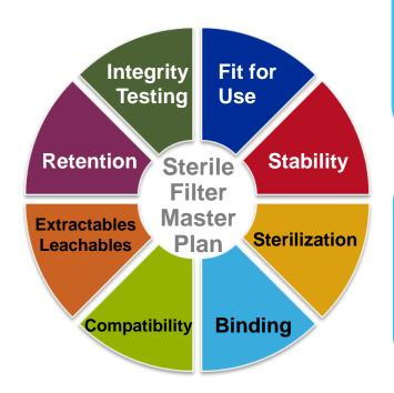
"pH and viscosity of the material to be filtered, flow rates, pressures, temperature, compatibility of the material with the filter itself, and the effect of hydraulic shock are factors of production which can affect filter performance and which should be simulated during validation of filtration processes"
